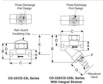
The Armstrong CD-33 is a disc style trap designed to control the trap's cycle rate. By reducing the cycle rate, the Armstrong CD-33 will have a longer service life than typical disc traps. This enhanced performance will ensure that maintenance time is minimized and steam costs are greatly reduced.
